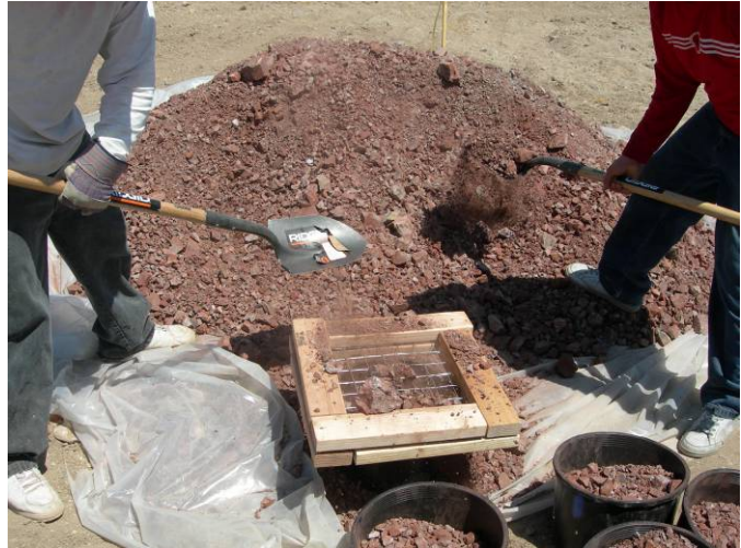
Image 4. Filling pots with the Arkose soil type. Note the red gravelly nature of the material.
